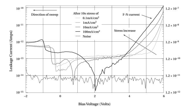
*Figure 1.* Pronin plot of gate oxide capacitor leakage current, voltage swept from 6V to –2V, 70Å oxide over well, no source or drain implants around capacitor.
